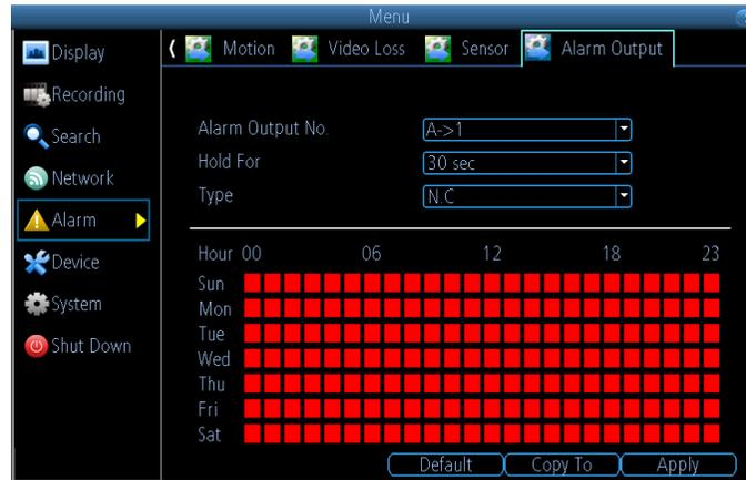
**Alarm Output No.:** Set the alarm output No. when triggering alarm sensor. 2 alarm outputs can be selected.
